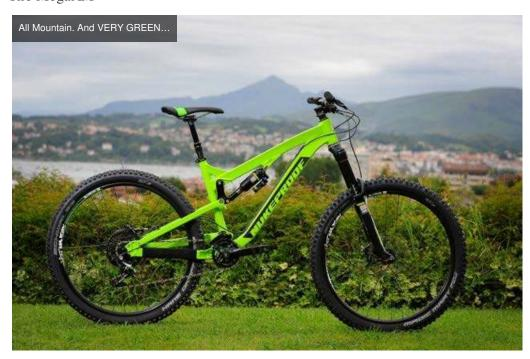
The Nukeproof AM is a beast of a bike - 160mm front and rear courtesy of a RockShox Monarch plus shock with a Pike fork, a  $1 \times 11$  SRAM XO groupset and Avid Guide brakes means that it could quite happily get me into - and out of - a whole heap of trouble, provided I have the confidence and chops to let it. It seems I
